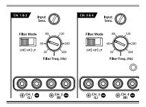
"Filter Mode" Control: The M400/4 employs a 12dB per octave filter for each pair of channels (one filter for channels 1&2, another filter for channels 3&4 and a third filter for channels 5&6). Each of these filters can be configured independently into one of two filter types or defeated completely by way of the threeposition "Filter Mode" switches:
