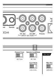
If you wish to send four discrete channels into the M400/4, simply use all four inputs and set the "**Input Mode**" switch in the "4 Ch." position.
