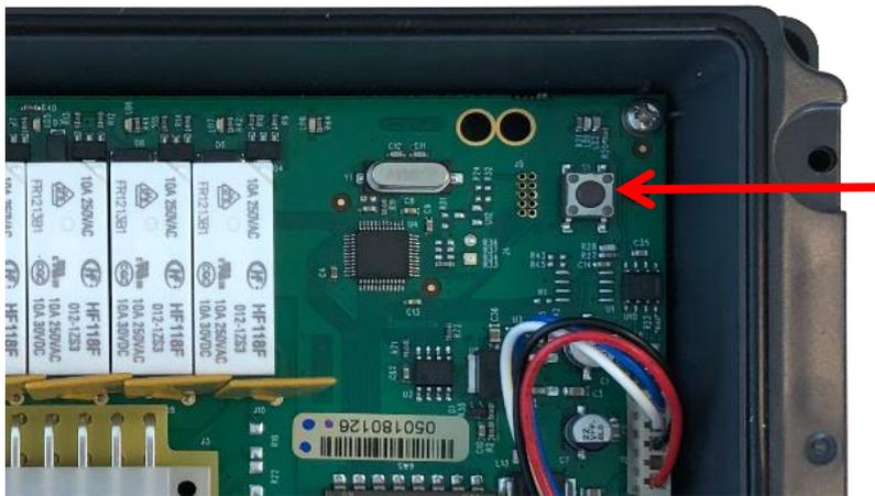
Follow the below steps to manually control each relay. To use manual override the Contact 6 must have 12V network power.
