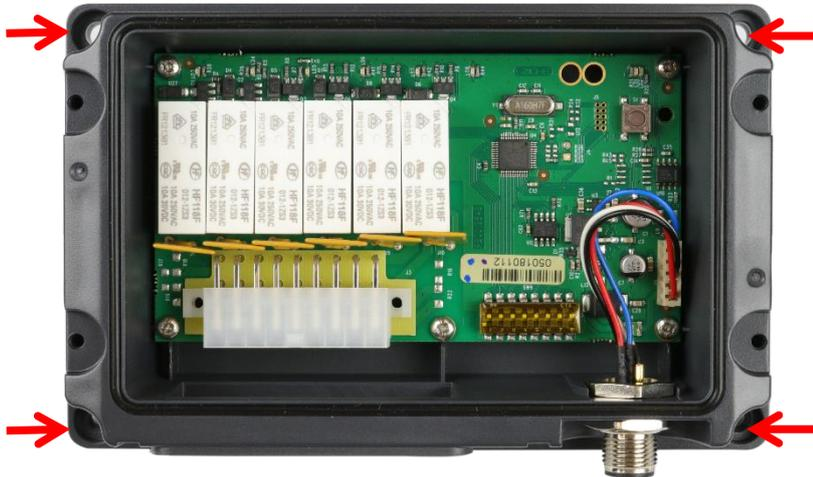
1. Remove the Contact 6 top cover and locate the 4 mounting screw locators as shown above.
