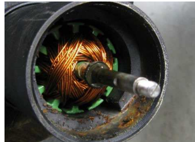
FIGURE 4 (Water damage to the lower unit)
