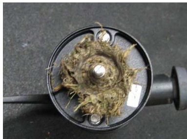
FIGURE 3 (Weeds caught behind propeller)
