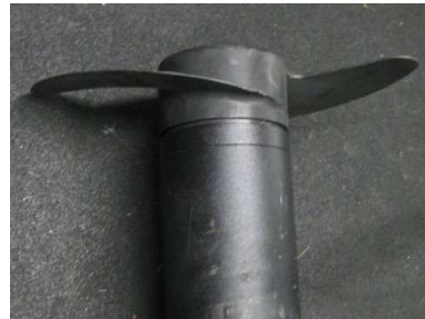
FIGURE 2 (Lower unit and prop with debris)
