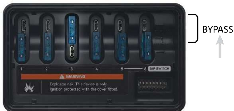
Fuse in Bypass Position
