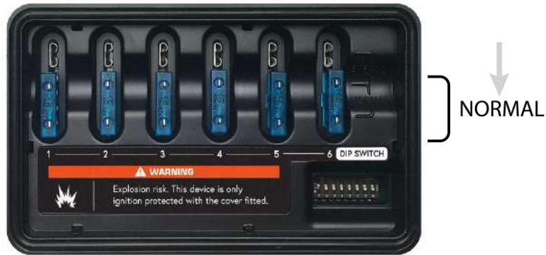
Fuses In Normal Operation
