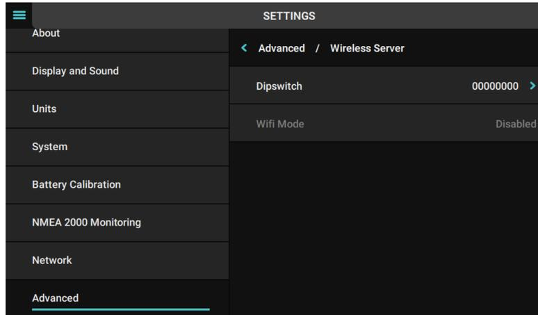
2. Enter the dipswitch as assigned in the CZone configuration, which should be different to the Touch 7 (Display Interface) dipswitch and press Save
