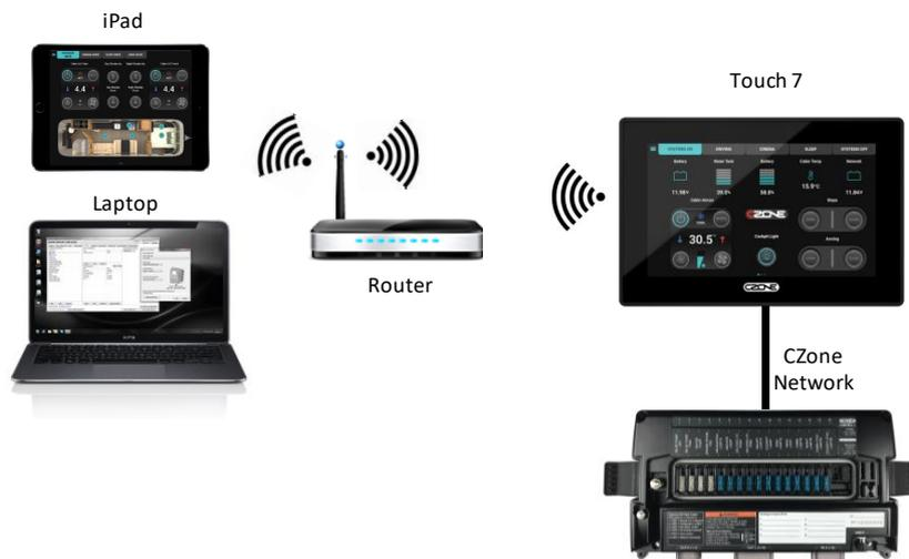
Figure 5. Client Mode Wireless Example
