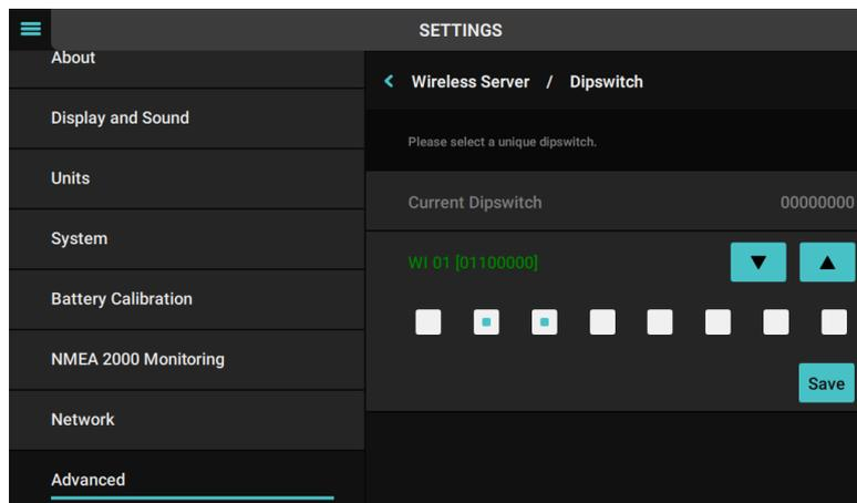
3. After Dipswitch is set, select the desired WiFi Mode. Refer to 2.5 for detail on each mode (note: select 'Disabled' to configure the device in Wired Client Mode. The WiFi will be disabled).
