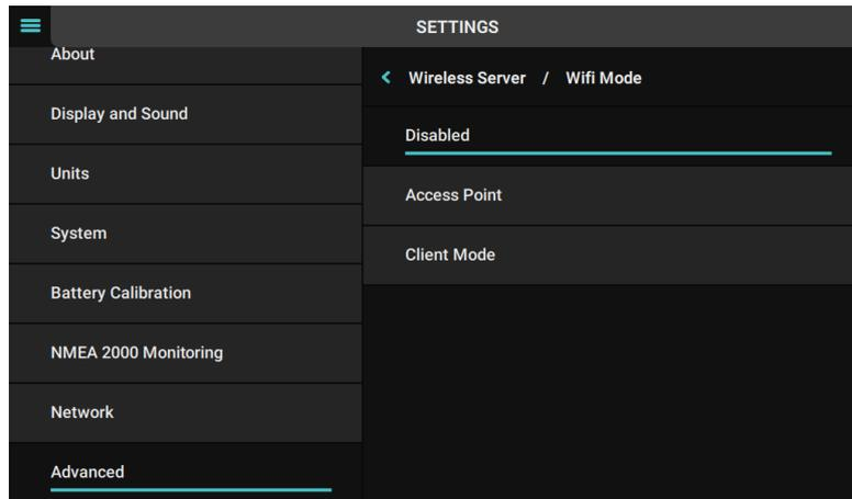
4. If Access Point is enabled the WiFi SSID and password will be shown per below image. Use these credentials to connect iPad to the Touch 7 or laptop to the Touch 7 for sending favorites configuration files (.cfp) wirelessly from the Favorites Tool.
