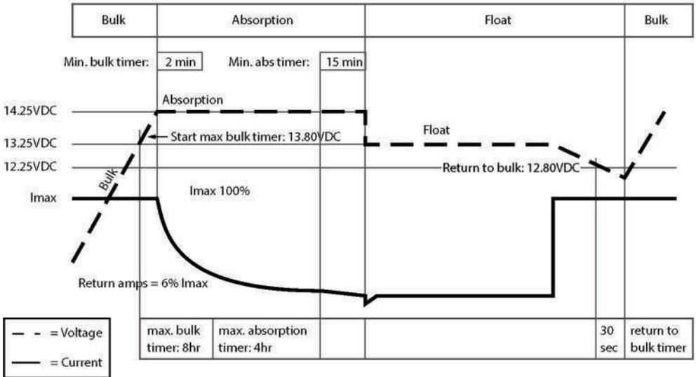
Figure 2. Typical charge characteristic (at 25°C / 77°F).
