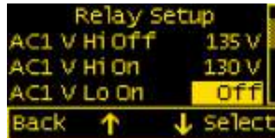
Relay Setup Screen with Relay Normal = On (Closed)
