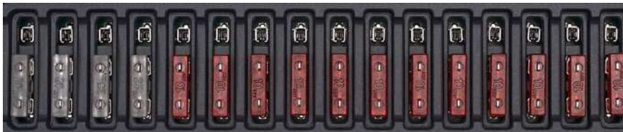
Figure 14. Fuses In Normal Operation
