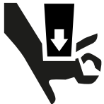
Caution: risk of crushing
