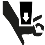
Caution: risk of crushing
