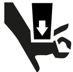
Caution: risk of crushing
