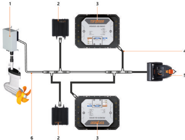
Fig. 45: Schematic arrangement of a TorqLink network with the 1976-00 accelerator lever
