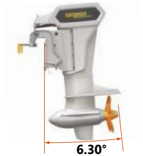
Fig. 51: Motor is tilted fully downwards
