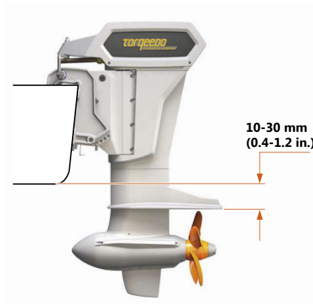
Fig. 33: Installation position
