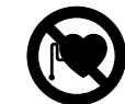
Persons with cardiac pacemakers or other medical implants must maintain a distance of 50 cm to the system.
