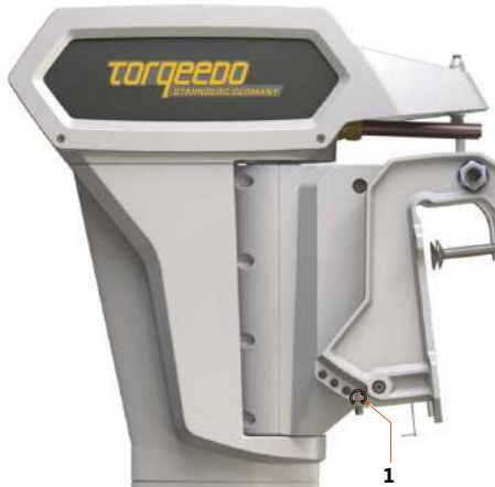
Fig. 40: Securing cotter pin for trim rod
