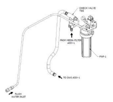
Figure 2.15: Freshwater Flush & Check Valve Assemblies
