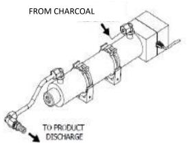
Figure 2.21: Ultraviolet Sterilizer
