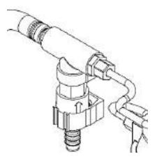
Figure 2.16: Check Valve (CV-1 & CV-2) Assembly
