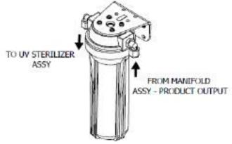
Figure 2.20 : Charcoal Filter (CF1 & CF2) assembly
