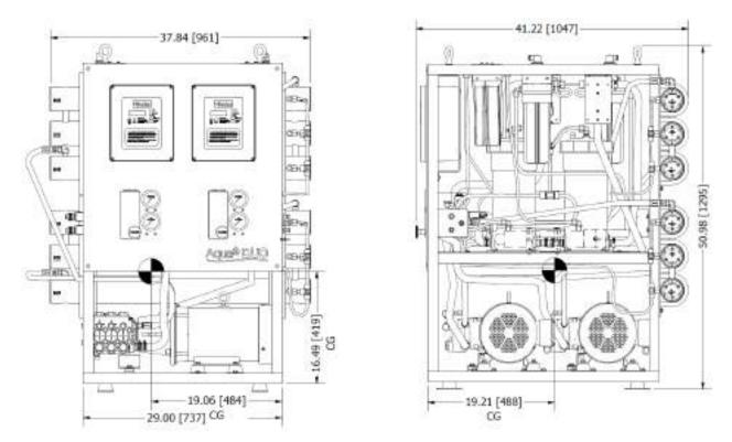
Figure 1.1: 4400 & 5800 GPD RO System Dimensions
