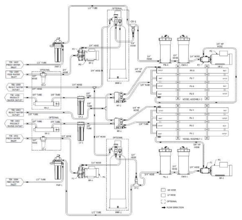
Figure 2.6: Piping and Instrumentation Diagram 4800-6200 GPD
