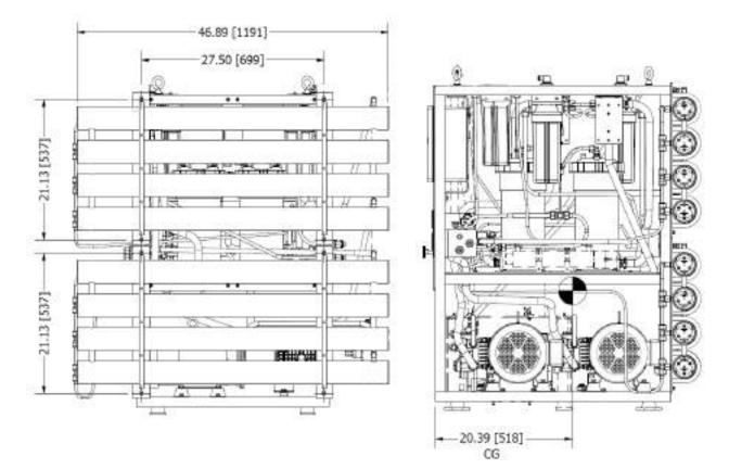
Figure 1.2: 5200 & 6800 GPD RO System Dimensions
