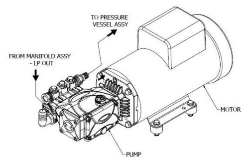
Figure 2.22: High Pressure Pump and Motor Assembly
