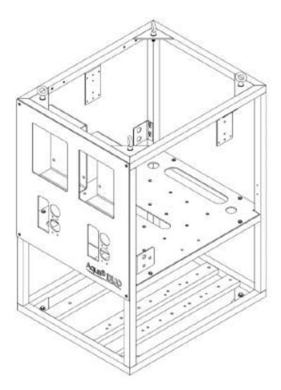
Figure 2.13: Main frame Assembly
