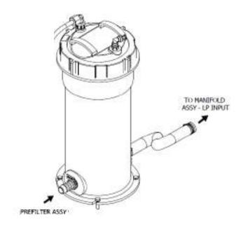
Figure 2.18: Oil & Water Separator (OWS-1 & OWS-2) Assembly
