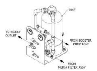
Figure 2.12: Optional Media Filter Assembly (MMF-1 & MMF-2)
