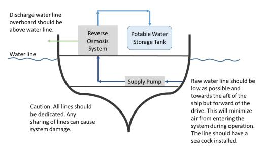
Figure 2.2: RO System Above Water Line
