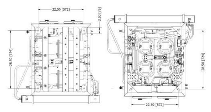
Figure 1.3: Mounting and Lifting lugs Dimensions of RO System
