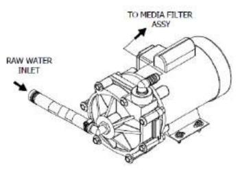
Figure 2.17: Boost Pump Assembly (BP-1 & BP-2)
