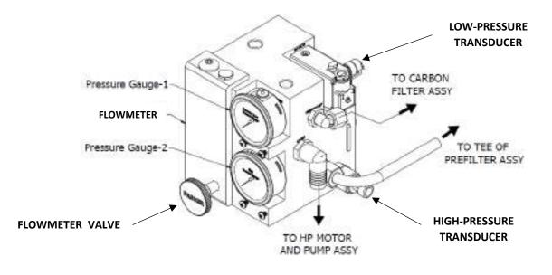
Figure 2.23: Manifold Assembly
