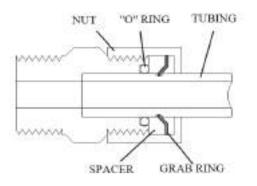
Figure 2.29: Tubing Fitting Internals
