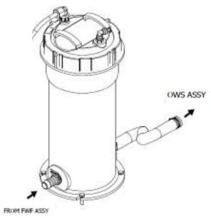
Figure 2.19: 5-Micron Prefilter Assembly
