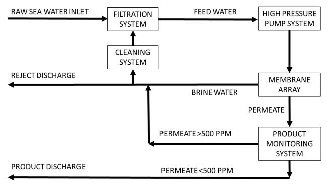
Figure 3.2: Simplified Schematic of a RO System
