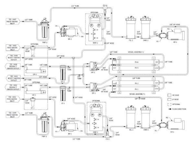
Figure 2.4: Piping and Instrumentation Diagram 2800-3600 GPD
