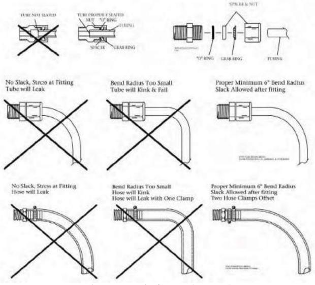
Figure 2.28: Hose & Tube Connection Instructions
