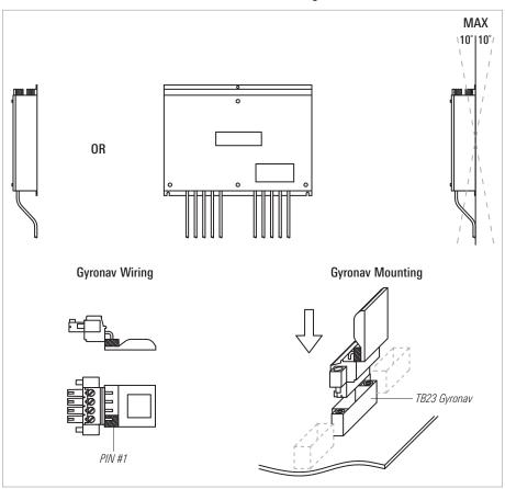
In a vertical mounting, the Course Computer is oriented horizontally on a vertical surface such as the bulkhead.
