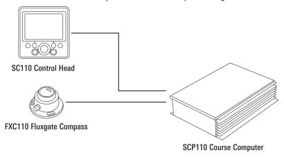
700049-1 SC110 Autopilot for Outboard System Configuration
