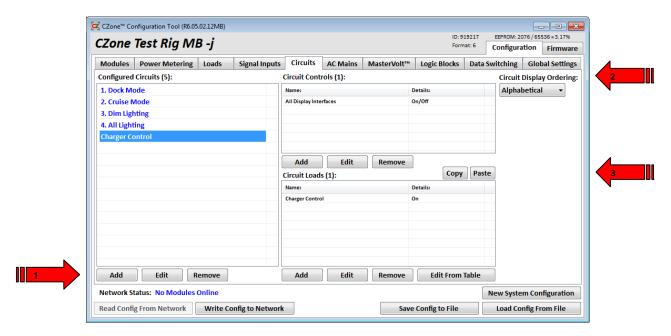
1. Go to the 'Circuits' tab. Under 'Configured Circuits' select 'Add'. Create a standard circuit, in this example called 'Charger Control'.
