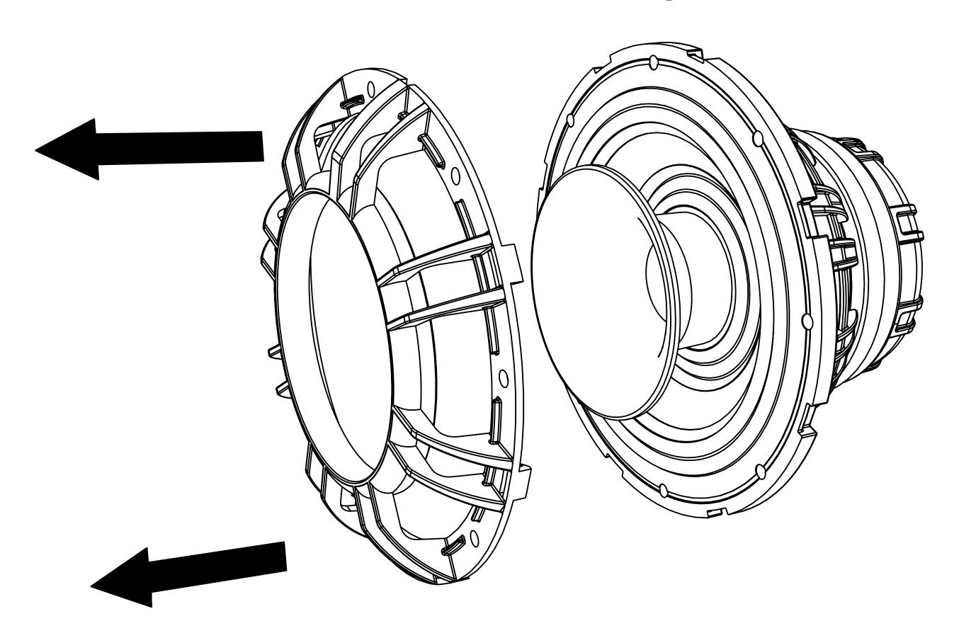
4. Unthread, remove and discard the installed horn.
