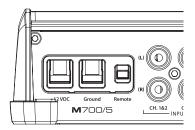
The M700/5's "+12 VDC" and "Ground" connections are designed to accept 4 AWG power wire. 4 AWG is the required wire size for this amplifier.
