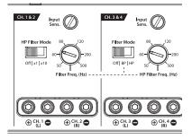
"Filter Mode" Controls: The M700/5 employs 12dB per octave filters for each pair of main channels (one high-pass filter for channels 1&2 and another high-pass / bandpass filter for channels 3&4. The Subwoofer Channel provides a low-pass filter with the option of 12dB or 24dB / octave slopes. Each of these filters can be controlled or defeated completely by way of the three-position "Filter Mode" switches in each Channel Section:
