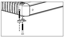
Lateral Mounting Feet are also included with your MHD600/4-24V to provide an alternative mounting option. Each mounting foot should be attached to the bottom of the amplifier by screwing the provided bolt into the bottom of the amplifier and up into the corner cap with the supplied 1/8-inch hex wrench. Next, using appropriate mounting screws (not included), secure the amplifier by its four Lateral Mounting Feet.
