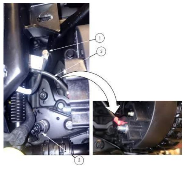
**6.** Mount engine block GND cable **(1)** on the engine block.
