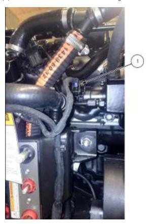
**15.** Connect the fuel pressure control valve (1).
