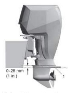
For high speed applications a higher mounting position, approx 25 mm (1 in.) above the boat transom bottom, might provide better performance.
