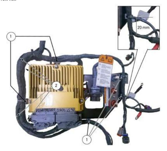
**1.** Fasten and secure wirig with clips (1).
