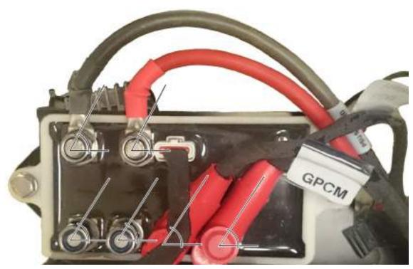
**1.** Mount the power cables at recommended angles as shown in picture above.
