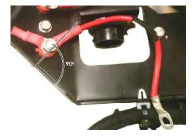
**1.** Mount the starter motor cable **(1)** in an right angle to the bracket edge.
