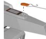
Fig. 14: Magnetic kill switch
