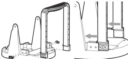
**NOTE:** The handle is keyed so that it only fits onto the base in one way.
